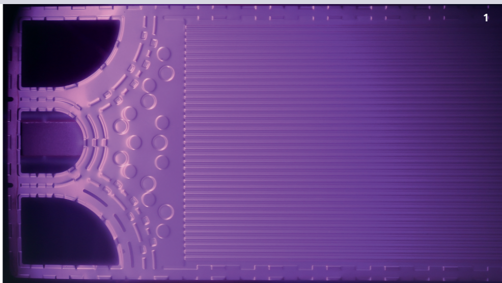
Functionalization of a metallic bipolar plate by means of plasma nitriding.
