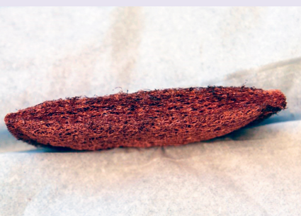
Coconut mat made from coconut fibers with copper coating.
