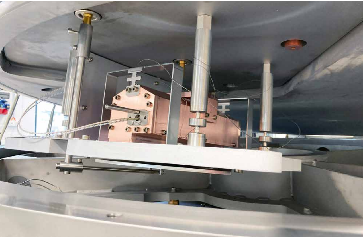
The evaporator system is constructed in the hybrid area of the S-ALD.
